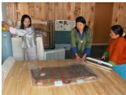
Figure 3. Purging the barrier film with nitrogen
