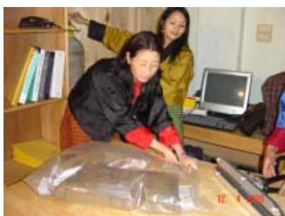
Figure 2. Purging the bag with nitrogen
